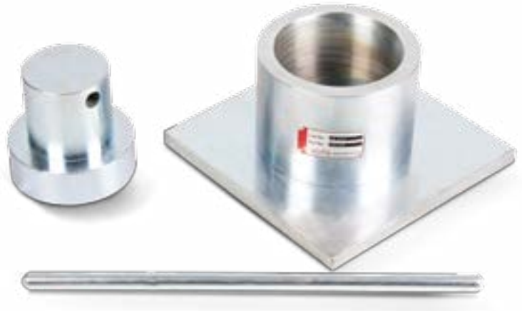
Aggregate Crushing Value (AG-210)
