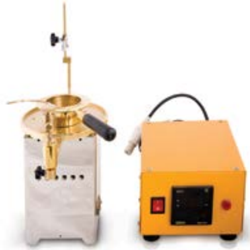
Flash Point Apparatus (A-470)
